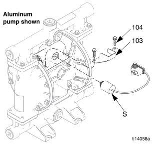
2. Use the screw provided to attach the reed switch just behind the air inlet. Remove the muffler, if needed, for easier access. Rotate the air inlet fitting as needed so the wrench flat clears the reed switch.
