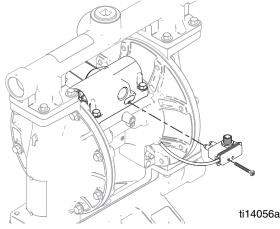
3. Connect the DataTrak cable to the 5-pin connector on the reed switch. Reconnect the air line to the motor.
