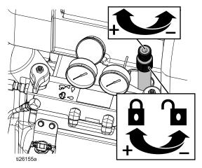
Component A and B outlet pressures will be higher than the hydraulic set pressure, depending on the model. Component A and B (GA, GB) pressure may be viewed on the pressure gauges or the ADM.  Check fluid pressure gauges (GA, GB) to ensure proper pressure balance. If imbalanced, reduce pressure of higher component by slightly turning PRESSURE RELIEF/SPRAY valve for that component toward PRESSURE
