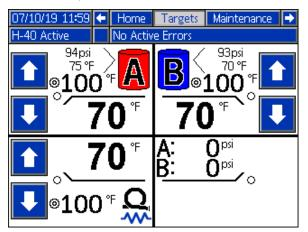
**NOTE:** Hose Resistance Mode controls the average fluid temperature of the A and B fluid. Set the hose temperature set point halfway between the A and B temperature set points and adjust as needed to achieve desired performance.
