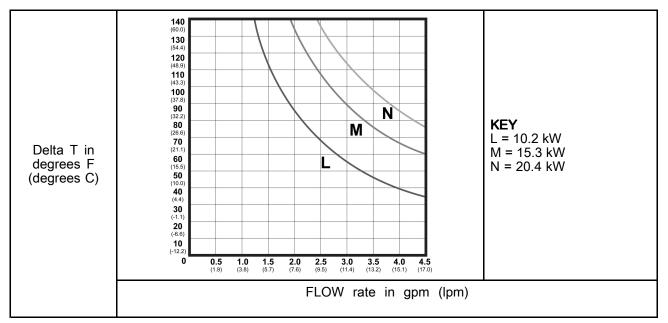
\* Heater performance data is based on testing with 10 wt. hydraulic oil and 230V across heater power wires.
