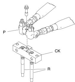
The Fusion AP gun manifold is shown.
