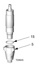
**13.** Disassemble intake valve. Be sure to remove o-ring (10).
