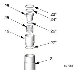
Component B (Resin) Pump: Install felt washers (21\*) into packing nut (19). Install retaining ring (22\*). Install packing nut handtight.
