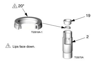
Models 246830 and 245970: Grease u-cup (20\*) and cylinder (2). Place seal installation tool (23\*) in cylinder. Place u-cup in tool with lips facing down. Be careful not to damage sealing edges of u-cup. Press u-cup in place with 7/8 in. deep-well socket (S). Remove socket and tool.
